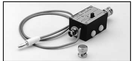
Model 6167 Guarded Input Adapter: Reduces effective cable capacity by driving the inner shield of the triax cable at Guard potential. For use with Models 220 and 224. 2-slot triax female to 2-slot triax male.
